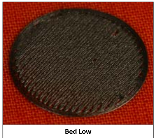
Stringy material or the lines don't connect completely to the outer circle: Bed low
